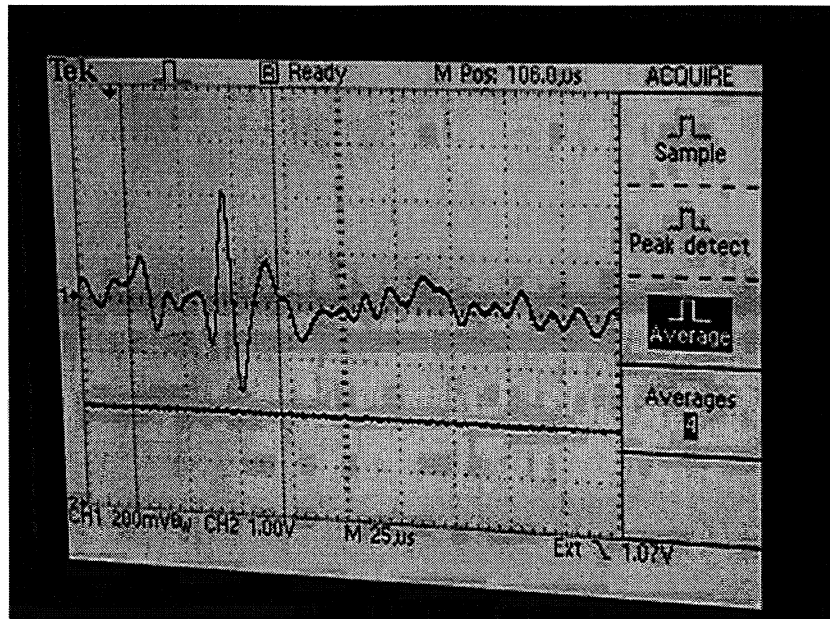
Figure 2.6.136 A_0 wave on copy paper moving at 2 m/s, detected with the self-mixing interferometer.
